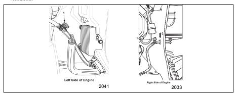
Figure 3–11 Fuel Shut Off Valves
